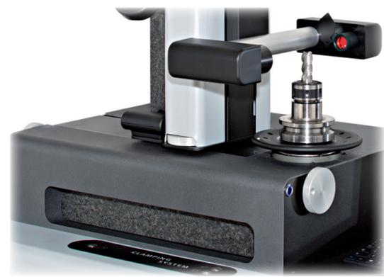
The base and the column, made of ground granite, are increased substantially in size over the previous generation model to guarantee and maintain maximum accuracy. The low coefficient of thermal expansion from this natural material allows the location of the machine directly in the workshop with no issue or concern in respect of accuracy and performance.
