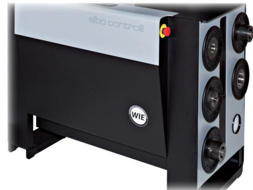
Great attention has been paid to the size and strength of the machine base which is totally produced from structural steel and is welded with both TIG and continuous welding. This concept allows the whole machine a very high stiffness the result of which guarantees high accuracy and rigidity.
