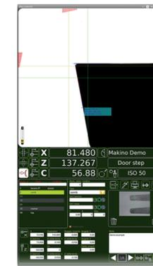
Also included for the first time is the capability for multi-measurement directly on the screen. So during tool inspection it is possible to make more than one measurement at a time on the same tool profile.
