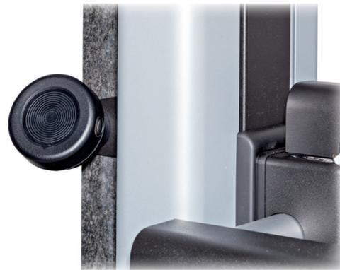
The ergonomic design and location of manual axis movements and controls allow for fatigue-free working. Simultaneous unlocking of both axes is activated by a single button. This operation for locking/unlocking of the axes is pneumatic. Bronze internal sectors act on the screw itself for both axes and have been designed to obtain high-precision fine adjustments.
