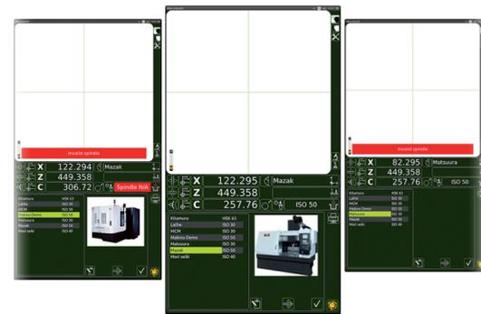
The new software also includes automatic recognition of the spindle via SP-ID (Spindle Identification System). This system allows the presetter to identify each spindle cartridge as it is loaded and suggest the correct machine origins, whenever the spindle is changed.
