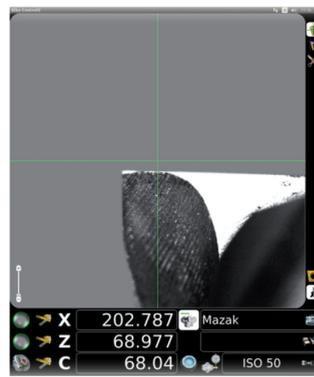
New electronics: a powerful PC running Ubuntu 14,04 LTS for the integrated management and control of the all the functions of measurement/tool inspection, machine origins and tool tables. Ease of use thanks to the integrated touch-screen.
