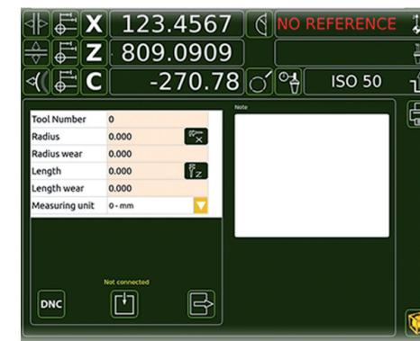
Also included is DNC connection software that allows the transfer of the tool offset data directly into the tool table of the Numerical Control (depending on CNC controller capability).
